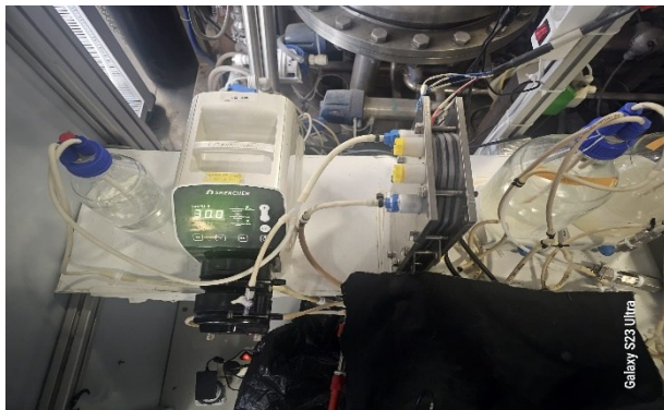
Figura 2.3 - Pila A, pompa Shenchen.
