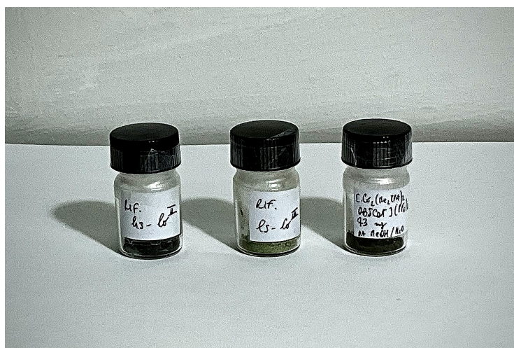
Figure 1.10: Powder samples of [\text{Co}(\text{Me}_n\text{tpa})(\text{diox-S-diox})\text{Co}(\text{Me}_2\text{tpa})](\text{PF}_6)_2 \cdot \text{MeOH} , where LS sample is in the center; the SCO sample is on the right and the HS sample is on the left.
