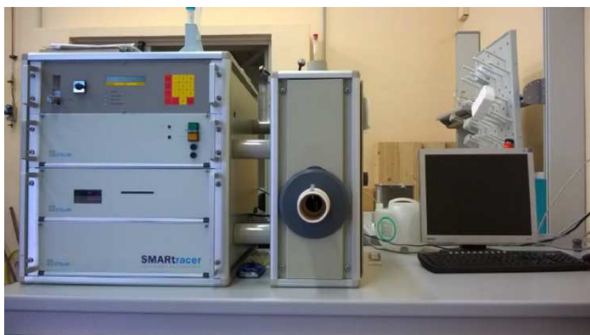
Figure 5.4: SMARtracer Relaxometer (Stelar s.r.l, Mede, Italy) used for the low-frequency measurements in Milan.
