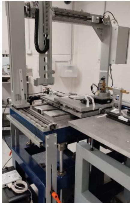
Figure 2.6: Remote positioning system for sample manipulation during irradiation.
