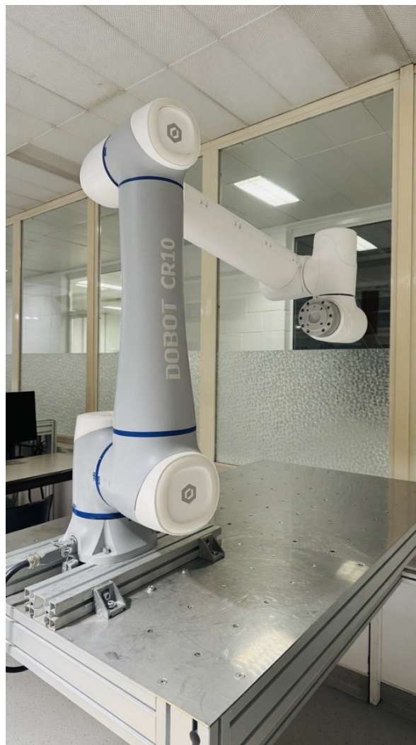
Figure 3.1. Dobot CR10 collaborative robot used in the experimental setup
