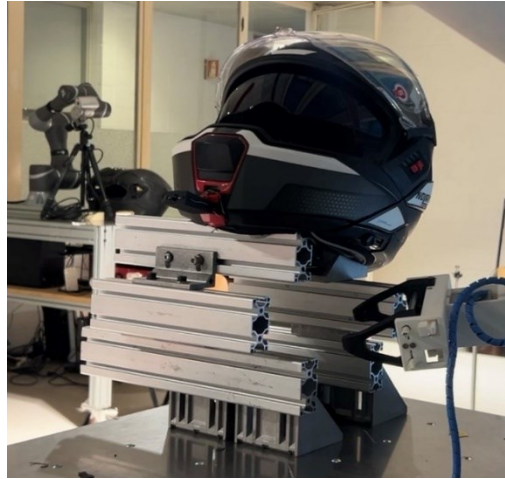
Figure 3.5. Helmet A used for testing the main visor, internal sun visor, upper air vent, and chin mechanism
