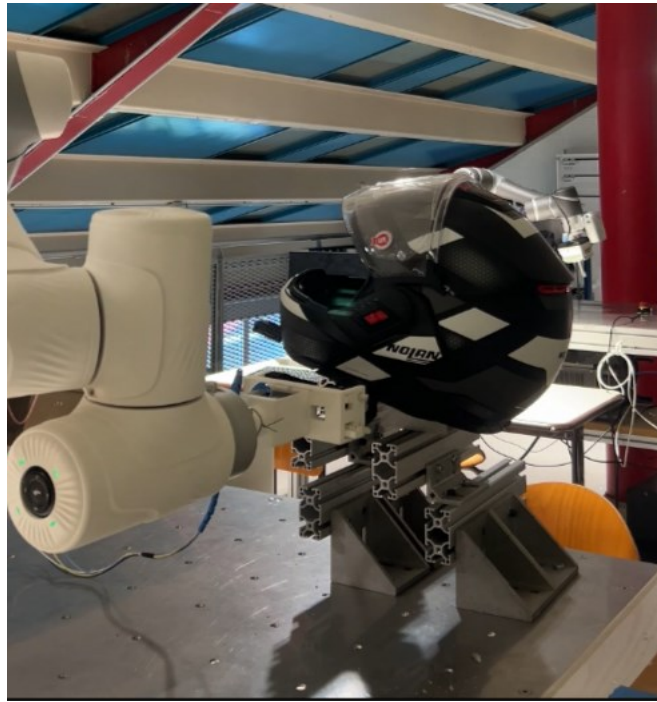
Figure 4.2. Robotic functional test configuration for the internal sun visor of Helmet A
