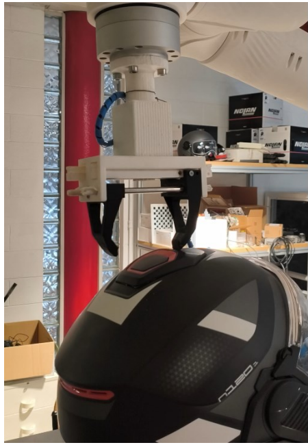
Figure 4.3. Robotic functional test configuration for the upper air vent of Helmet A
