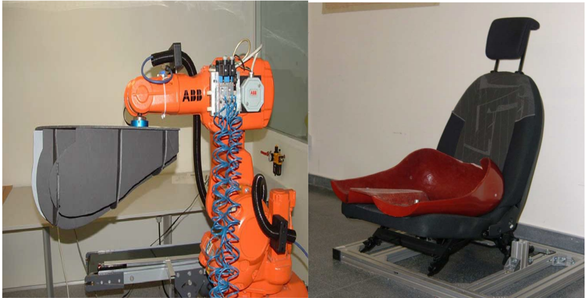
Figure 1.5. Industrial robot and test dummy used for automated anthropomorphic seat testing
