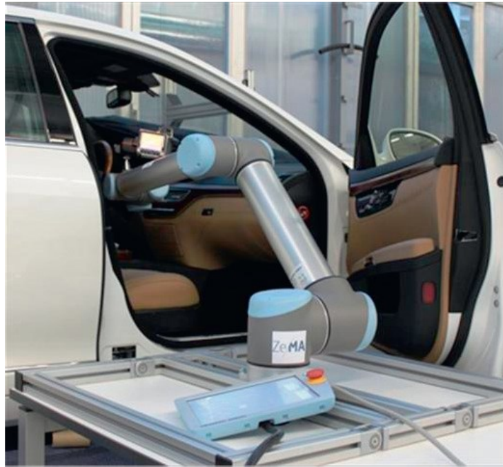
Figure 1.6. Collaborative robotic system for automated automotive water-leak inspection
