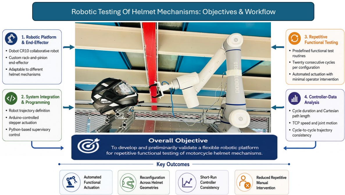
Figure 2.1. Overview of the proposed robotic testing system: objectives and workflow
