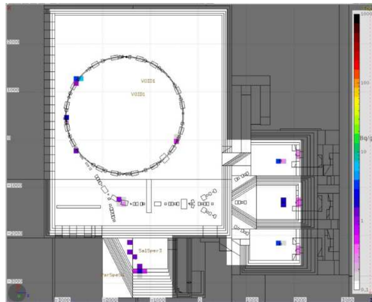
Figure 5.11: Visualization of the USERBIN-actomass in the x-z plane with y=-200 , for a Carbon ion beam at maximum energy and intensity.
