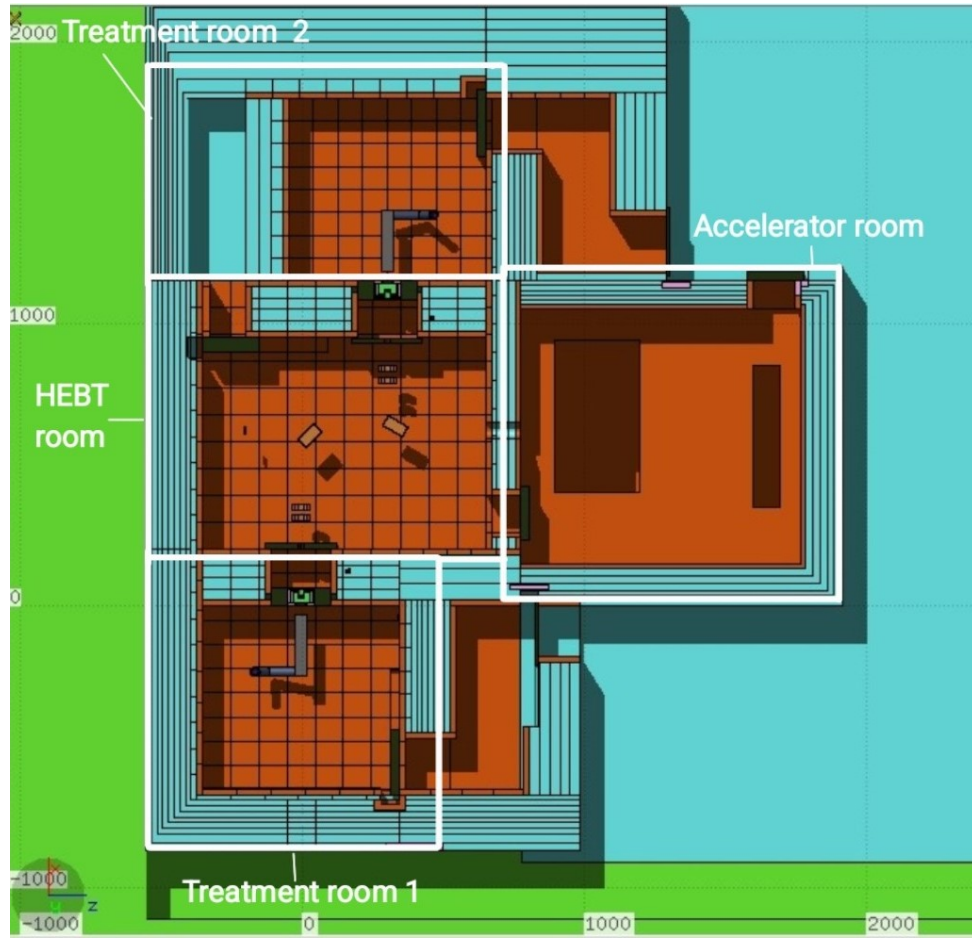
Figure 7.2: 3D representation of the BNCT facility, cutting plane x-z at y=0 , highlighting the rooms that compose it.
