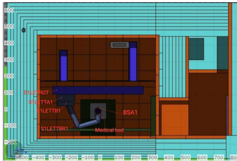
Figure 7.4: 3D representation of Treatment Room 1, cutting the y-z plane at x=-500 .
