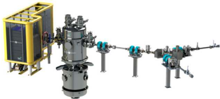
Figure 1.11: Tandem accelerator with source (on the left) and beamlines.
