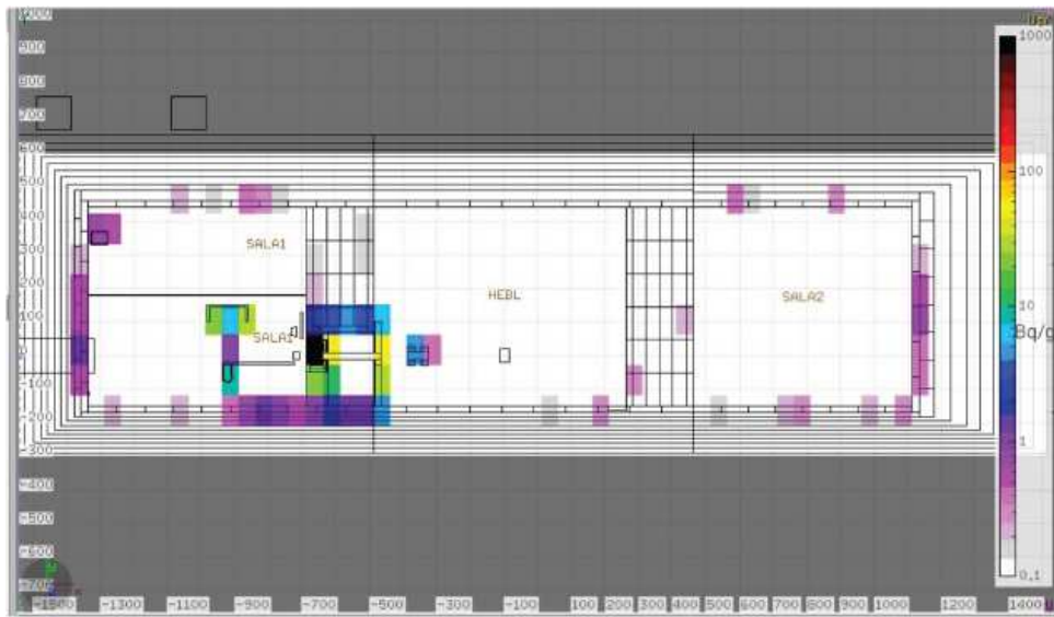
Figure 7.8: Visualization of the USERBIN-actomass in the x-y plane with z=0 .
