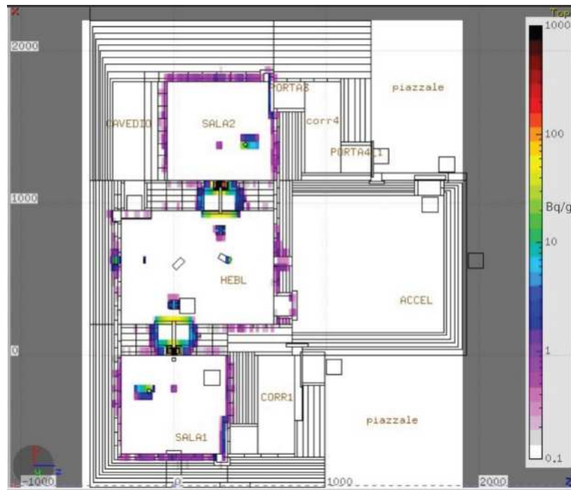
Figure 7.5: Visualization of the USERBIN-actomass in the x-z plane with y=0 .
