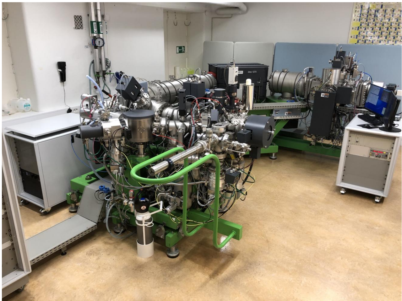
Figure 3 , The CAMECA IMS 1280-HR Secondary Ion Mass Spectrometer (SIMS) at the Swedish Museum of Natural History (NRM), used for Pb-Pb isotopic analyses.
