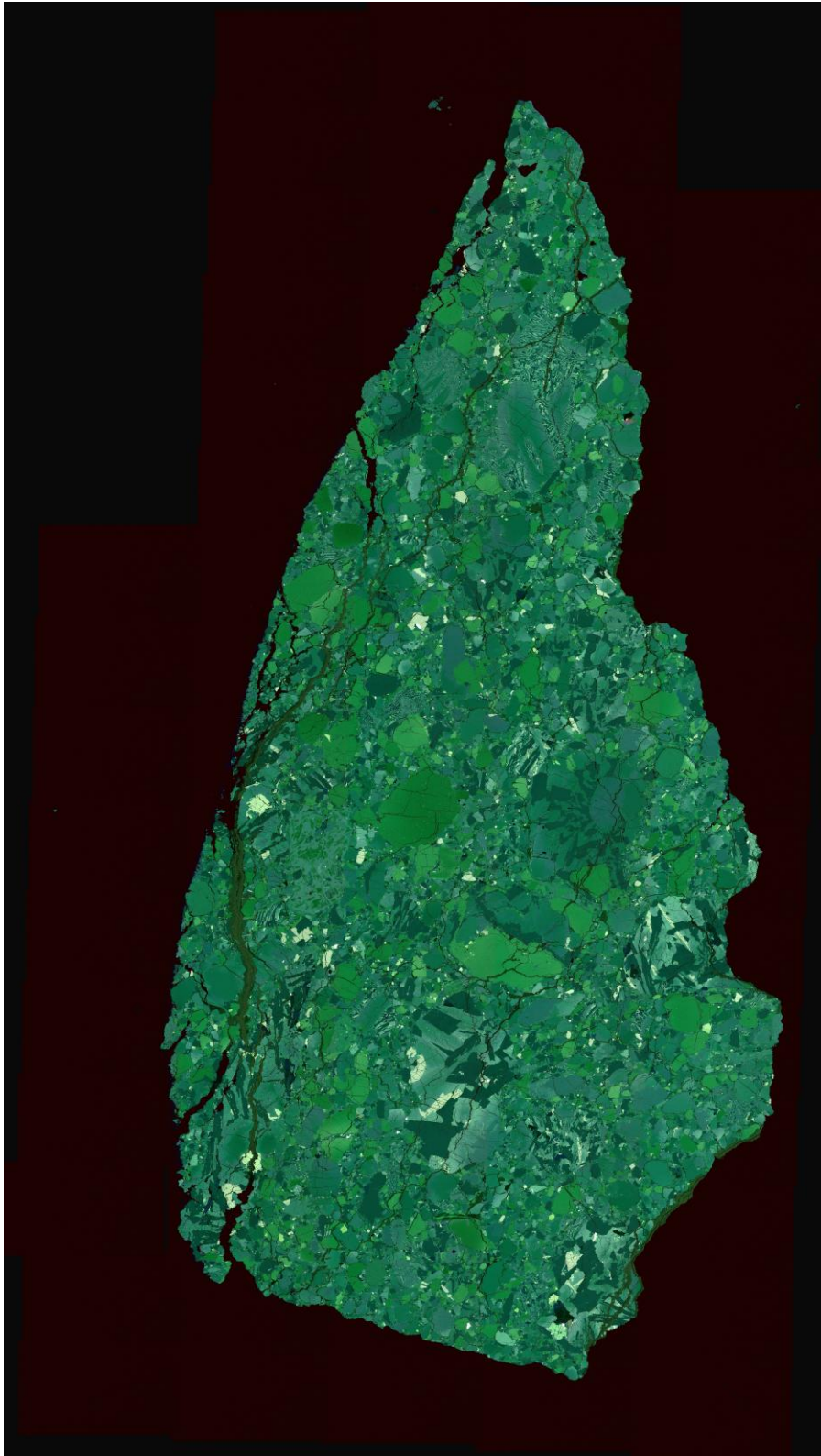
Figure 7 , Base EDS layer map used for the chemical analysis
