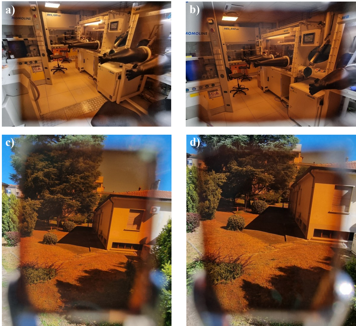
Figure 21. a,c) Photographs of the 140 nm device (Glass/ITO/MeO-2PACz/Perovskite/PCBM/BCP). b,d) Photographs of the 160 nm device.
