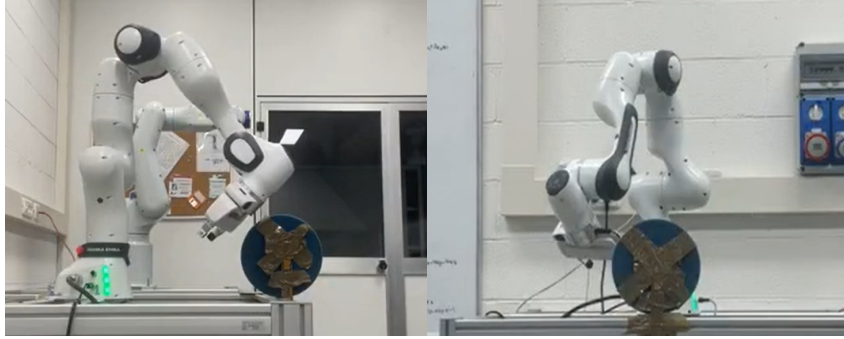
Figure 17: Initial position of the FR3 during the 3D case lab tests.
