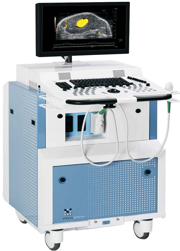
Figure 3.2. Vevo 2100 micro-ultrasound imaging system (VisualSonics, Toronto, Canada) used for transthoracic echocardiography. Image adapted from manufacturer's website
