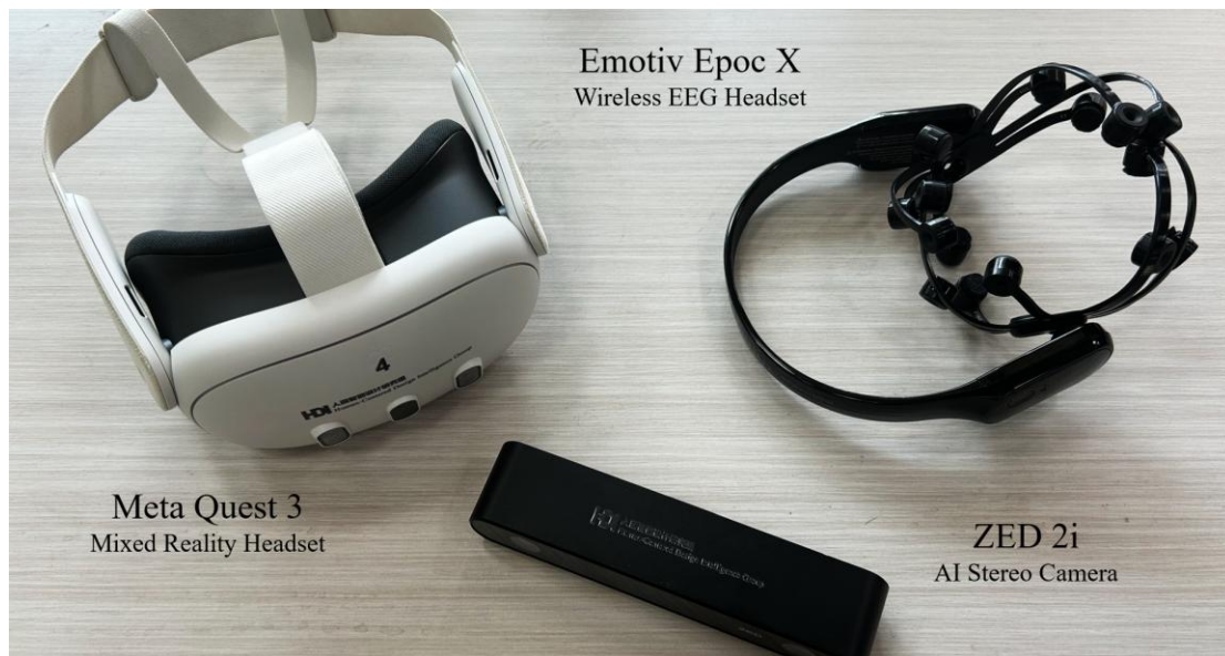
Figure 3.8: The experimental apparatus employed in the study, comprising the Meta Quest 3 Mixed Reality (MR) headset for virtual spatial simulations, the Emotiv EPOC X wireless Electroencephalography (EEG) headset for real-time neurophysiological data collection and the ZED 2i AI STEREO Camera. Source: [Author].
