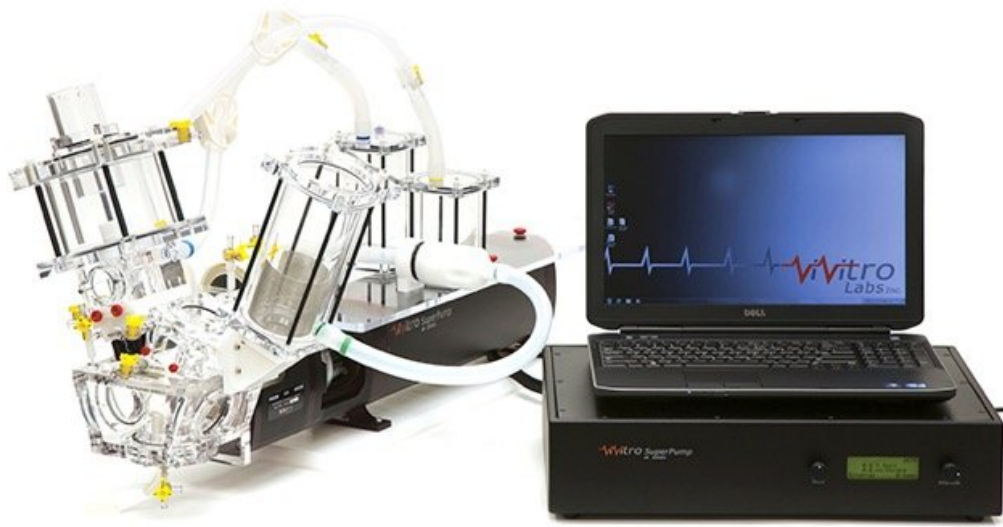
Figure 2.14: Illustration of the complete Vivitro Pulse Duplicator system (from Ref [17]).
