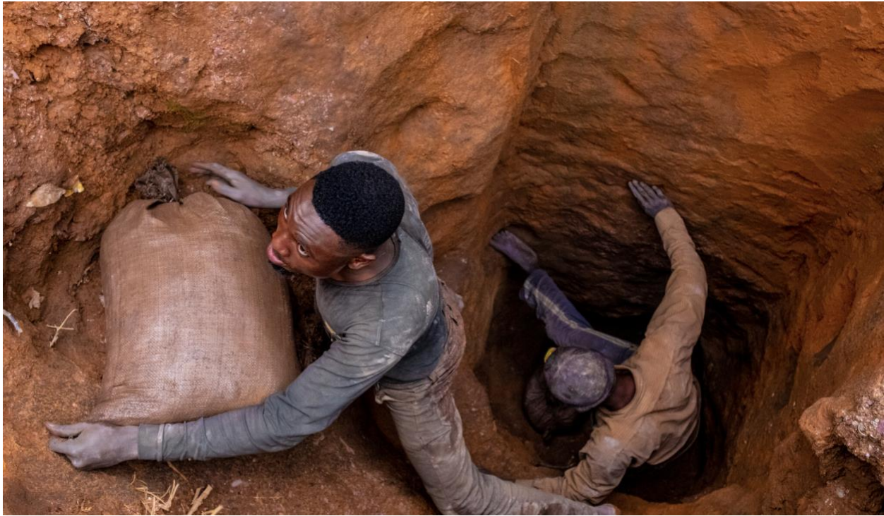
Artisanal miners peer up from the hand-dug shaft that poses a risk of collapse(Dorothee Baumann-Pauly,2022)
