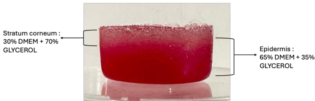
Figure 23: Composition of the two different layers of the skin mimicking AG/GEL hydrogel.
