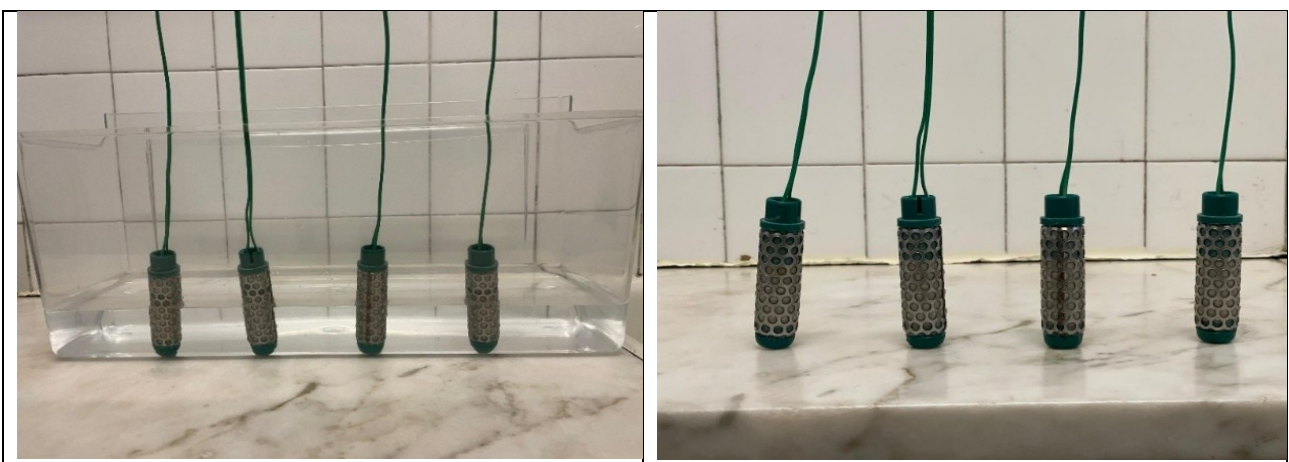
A) Day 1 (Morning): 30-minute partial immersion, followed by air-drying until the evening.
