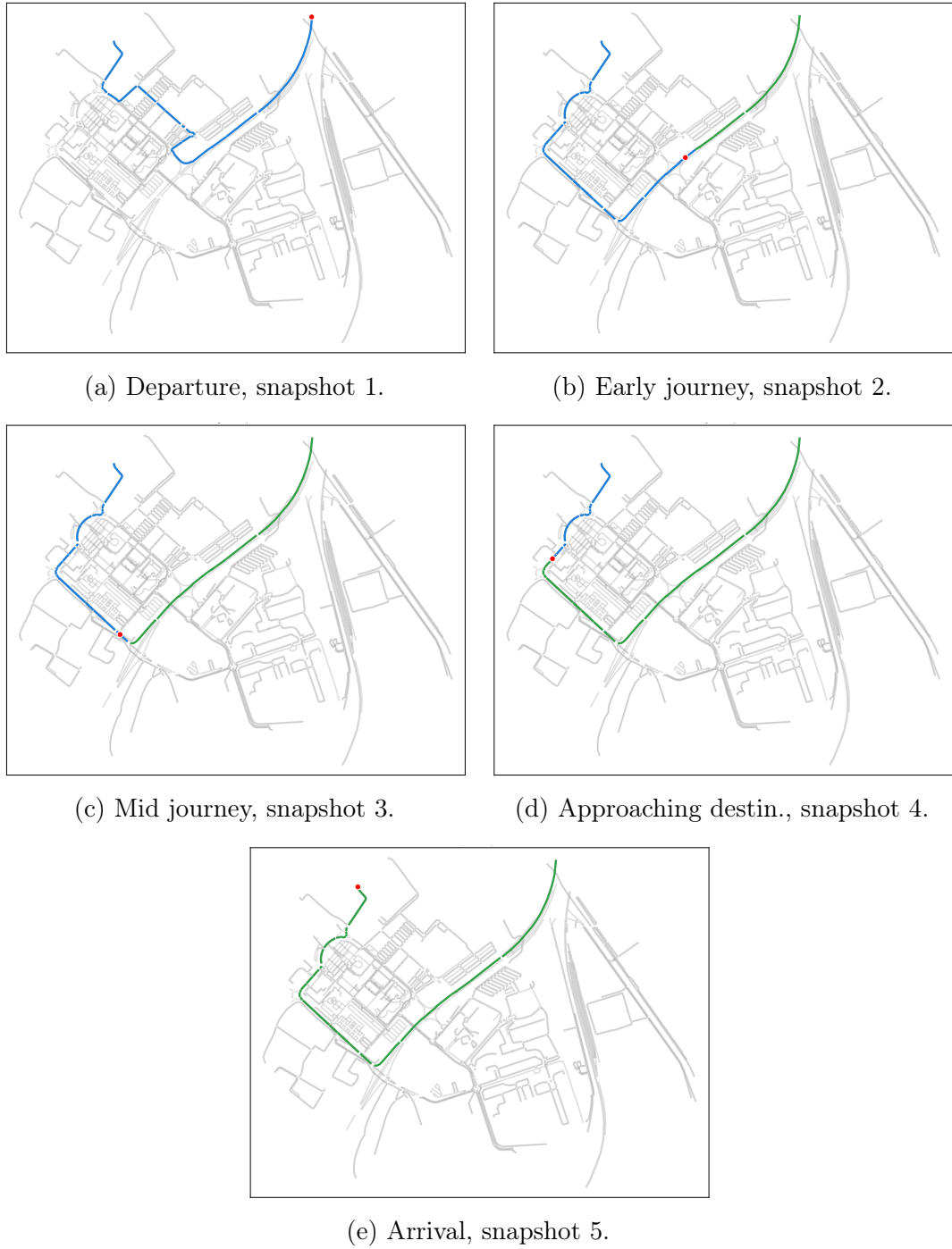
Figure 4.6: Five snapshots at time 350.5 s, 384 s, 422 s, 464 s, 506.5 s of the EGO vehicle's planned route (blue) on the Nave network, from departure to arrival. The route is progressively shortened and re-shaped as the vehicle advances and reacts to the live traffic state.
