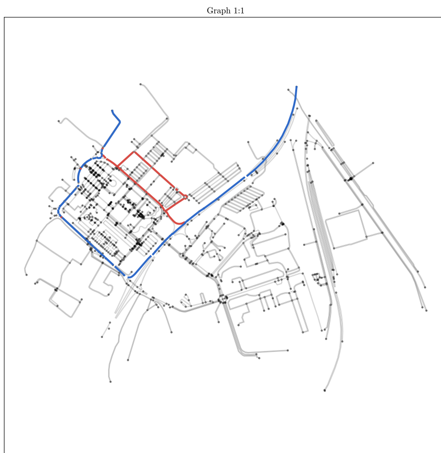
Figure 4.5: 1:1 topological graph of the Nave road network reconstructed with NetworkX. Grey: the full network; blue: the edges actually traversed by the EGO vehicle; red: the discarded paths.
