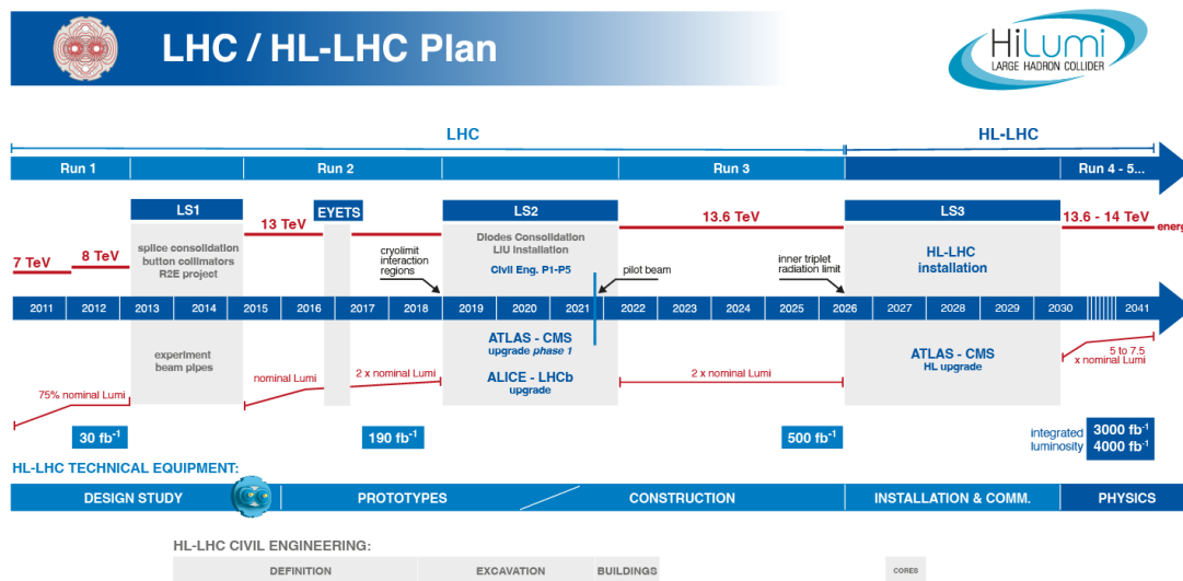
Figure 1.9: Timeline of LHC upgrades and modifications up to HL-LHC [12].
