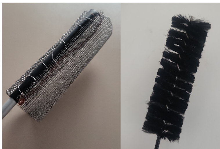
Figure 6: Stainless-steel mesh cathode (left) and carbon-brush anode (right) used in the AD-BES reactor.
