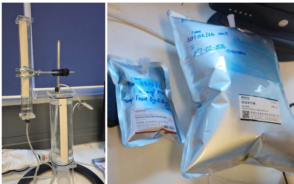
Figure 7 (left) and Figure 8 (right) respectively the water displaced system composed in two plexiglas tubes with graph paper tape on it and two different size aluminium foil gas sampling bags from AD (left bag) and AD-BES (right bag) from the same sludge period.
