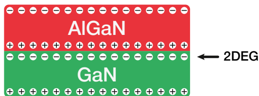
Figure 1.1: Cross-section of a GaN/AlGaN heterostructure showing the formation of a 2DEG.
