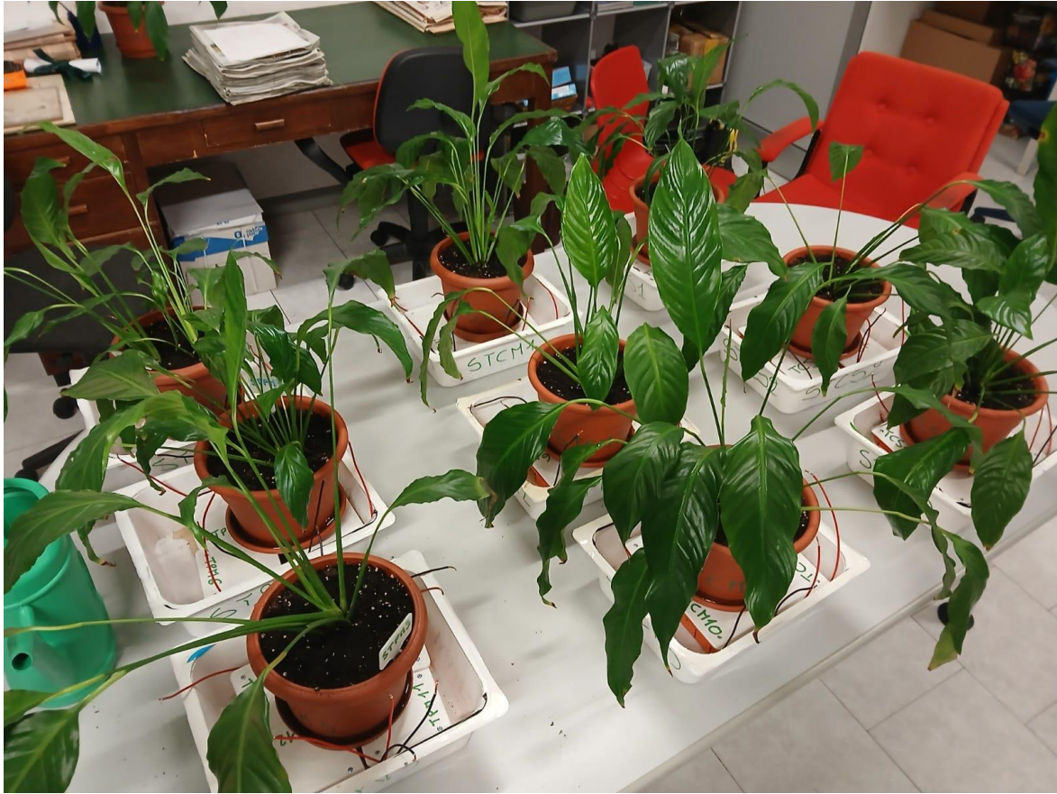
Figure 16: PMFCs with Spathiphyllum lanceifolium
