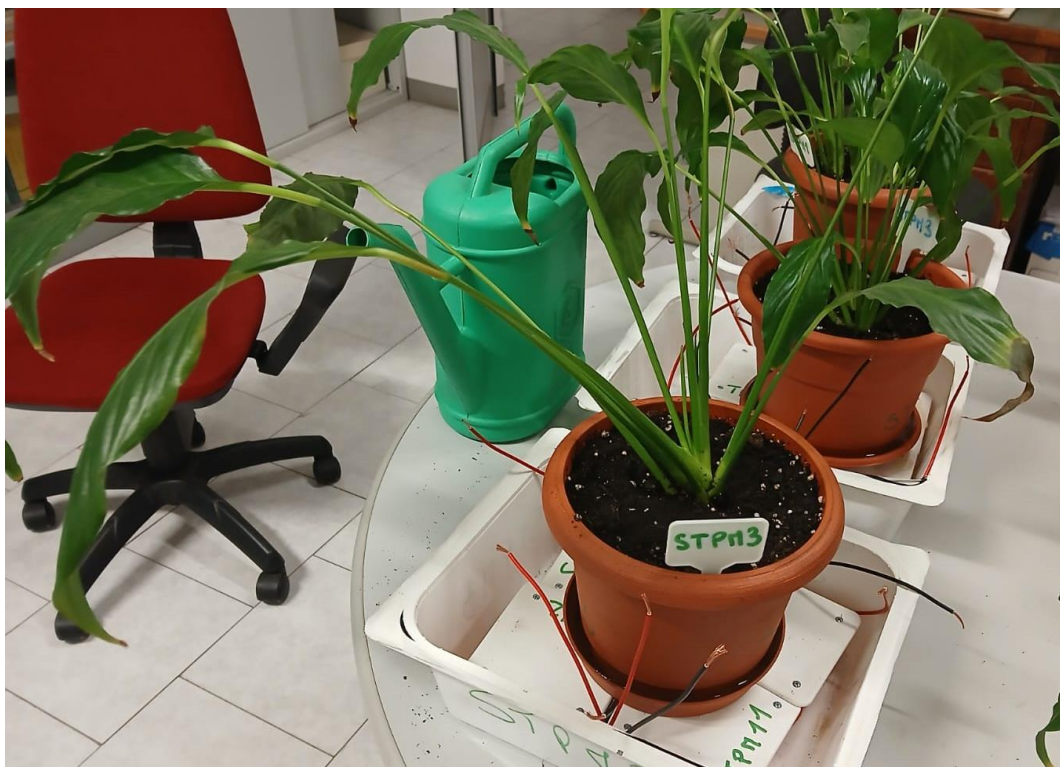
Figure 5: Spathiphyllum lanceifolium , as a plant-microbial fuel cells (PMFCs)
