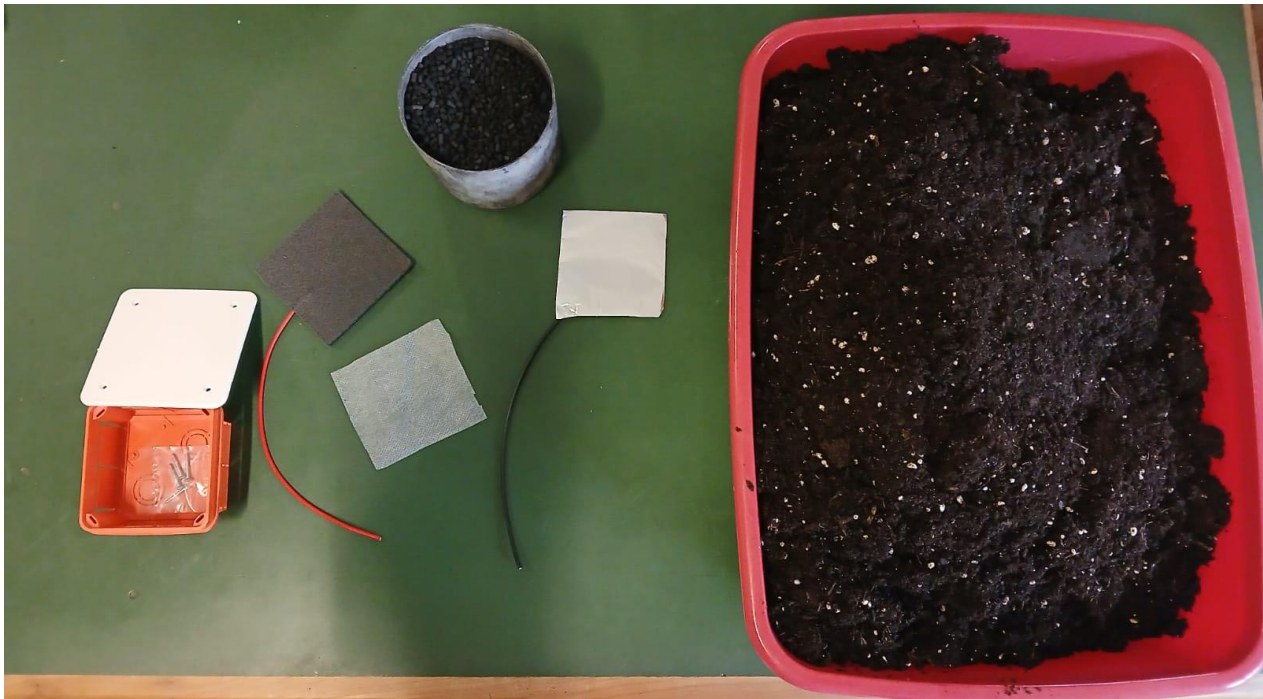
Figure 10: Cells components: derivation box, anode, non-woven fabric, carbon pellet, cathode and soil
