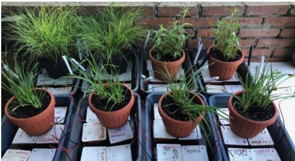
Figure 18: The 48 PMFCs of the Outdoor experimentation
