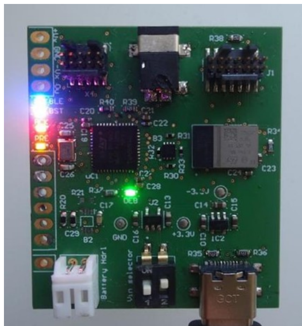
Figure 3.8: PCB at High Voltage Led ON
