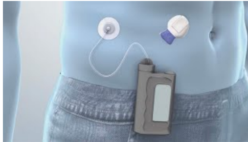
Figure 1.5: Conventional pump connected with CGM sensor [5]
