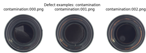
Figure 1.2: Example of defects on a bottle
