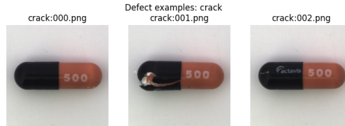
Figure 1.12: Test defected samples, class “Capsule”, defect “crack”
