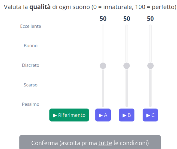
Figure 3.5: The MUSHRA interface designed for the experiment. The layout matches the example specified in ITU-R BS.1534-3.
