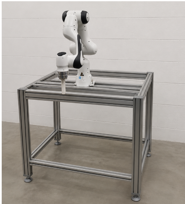
Figure 4.5: Emika Panda Robot with customized end-effector
