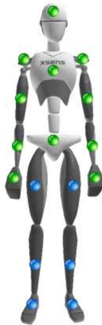
Figure 7.2: MVN suit configuration; green dots represent sensors placement, from [31].
