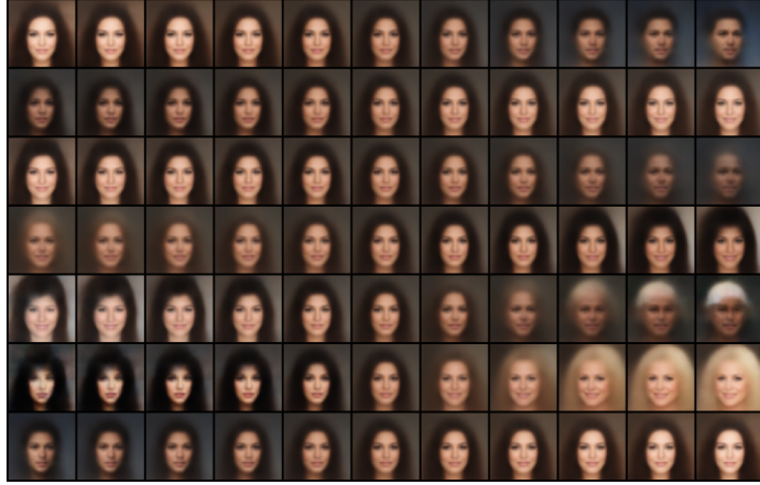
Figure 4.12: Attribute direction manipulations applied to a base encoding for the 60M RLT model trained for 100 epochs with 512 latent dimensions, rescale set to 1 KL annealing and free bits set at \tau = 0.1 . Each row corresponds to a different attribute, in order: Male , Smiling , Eyeglasses , Young , Bald , Blond_Hair , No_Beard . Each column display the base encoding plus \alpha \cdot \mathbf{v}_a , where \alpha varies linearly from -5 to 5 from left to right.
