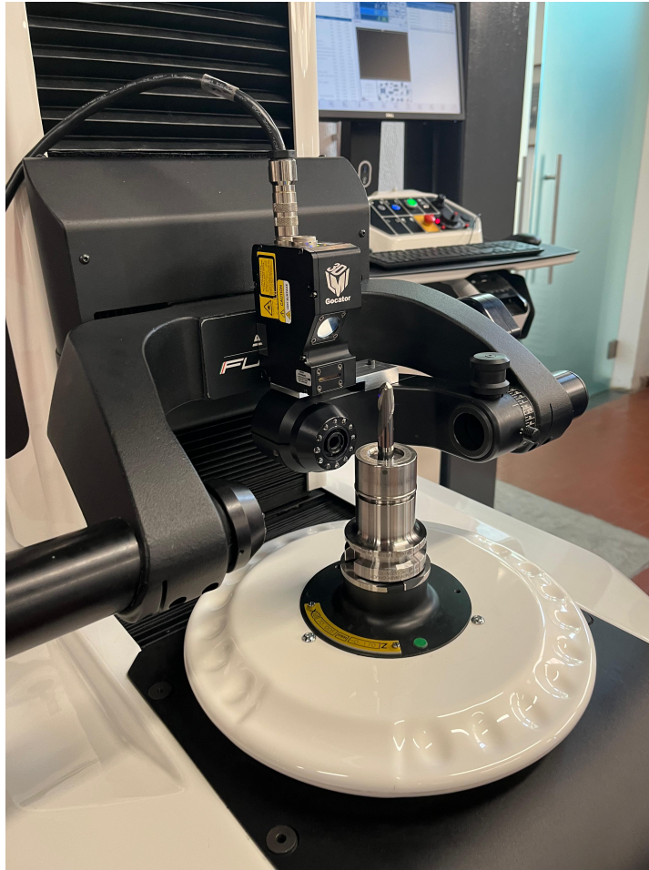
Figure 5.1: Laser triangulation sensor mounted on the Speroni machine.
