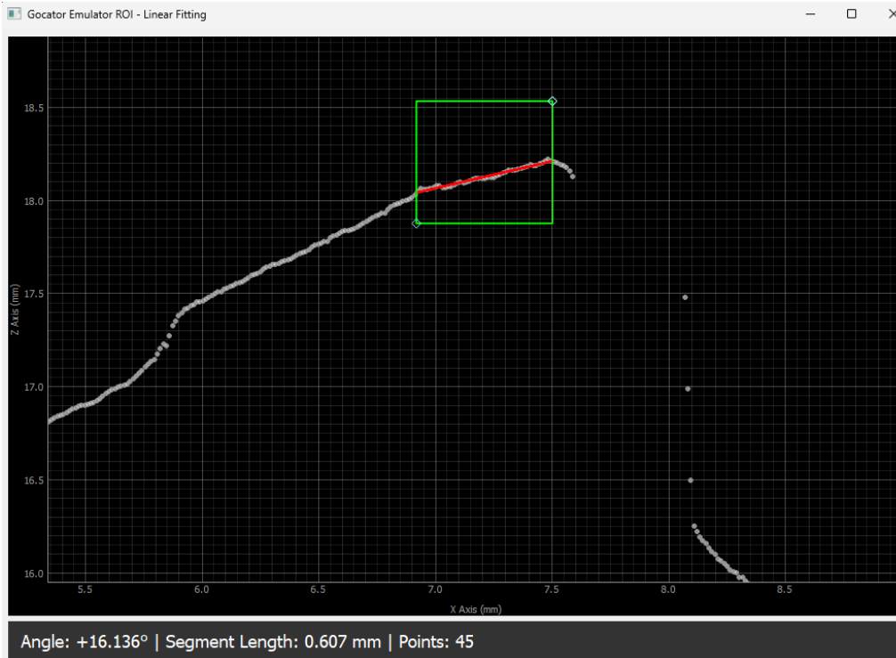
Figure 5.6: Successful angular and length measurement within a manually adjusted ROI.
