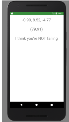
Figure 3.3: Using feature C_9 in real-time within the Android application. The figures in the first row represent the accelerations on the three axis, while the value in the second row is that of feature C_9 computed over the previous 128 samples. The third row indicates whether this value is above or below the predefined threshold.
