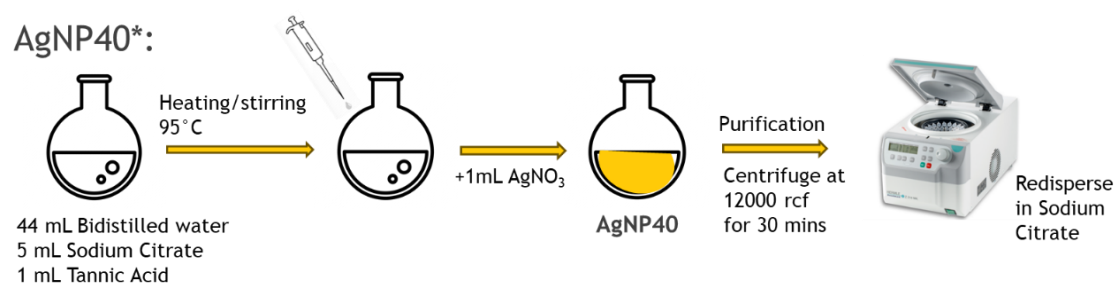
Figure 19 Scheme of the synthesis procedure for AgNP40 *Adapted from (17)
