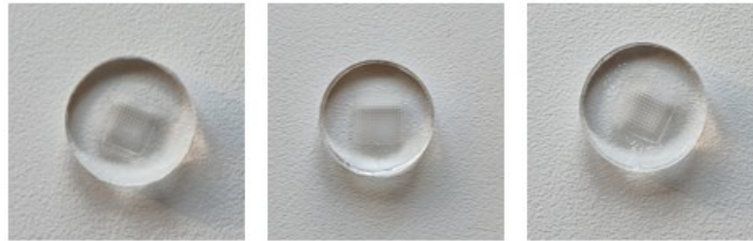
Figura 25 - Stampi MPatch TM Microneedle Templates 15x15 H600 (sinistra), 10x10 H600 (centro), 10x10 H800 (destra).
