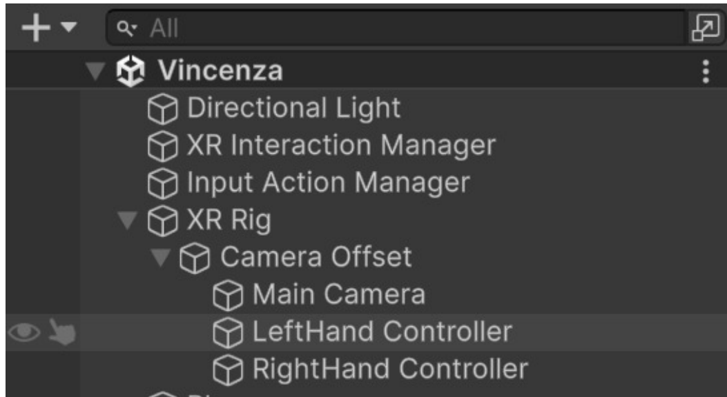
Figure 4.16: Hierarchy view in Unity after adding the XR Origin (VR) prefab.
