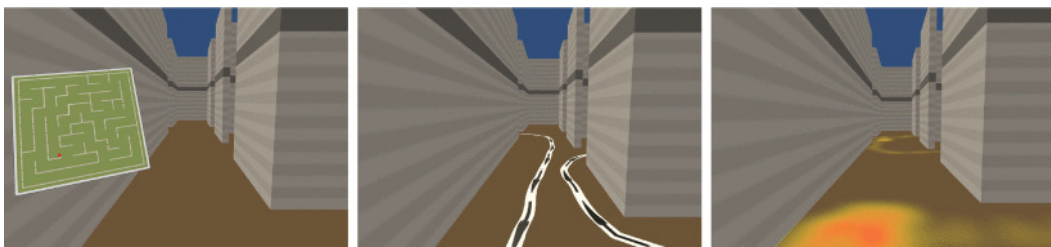
Figure 2.1: Three orientation aids in a maze-like VR scene: left-a corner mini-map; middle-a path trail; right-a visit-trace heatmap. The latter two are rendered directly in the main scene and therefore use a “breadcrumbs” approach to show path history [12].
