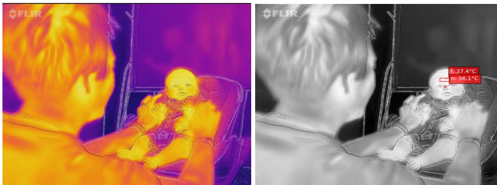
Figure 2. A visual example of the infant's raw ITI data and temperature extraction at the nasal tip and forehead regions of interest
