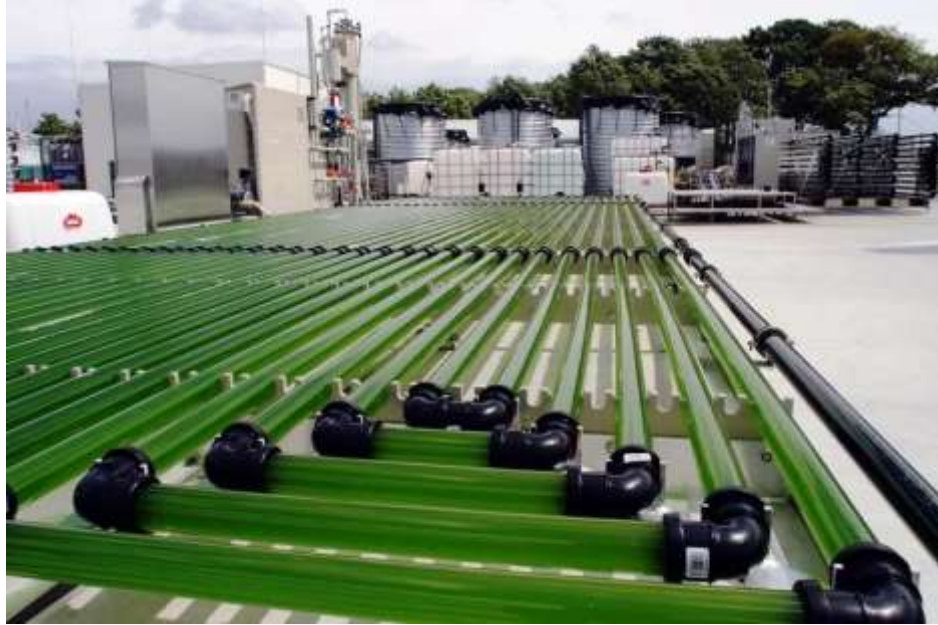
Figure 3: 6 Horizontal Tubular Photobioreactor Microalgae Cultivation System and Biorefinery [16]
