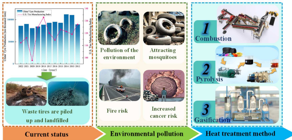
Figure 1.1: Current status of waste tires, environmental impacts, and main heat-treatment methods [2].
