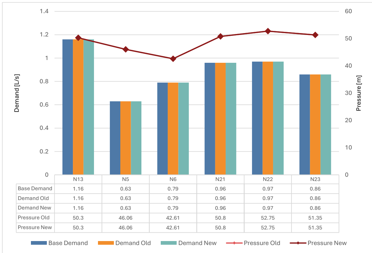
Figure 3-5 Initial condition (Old vs. New)
