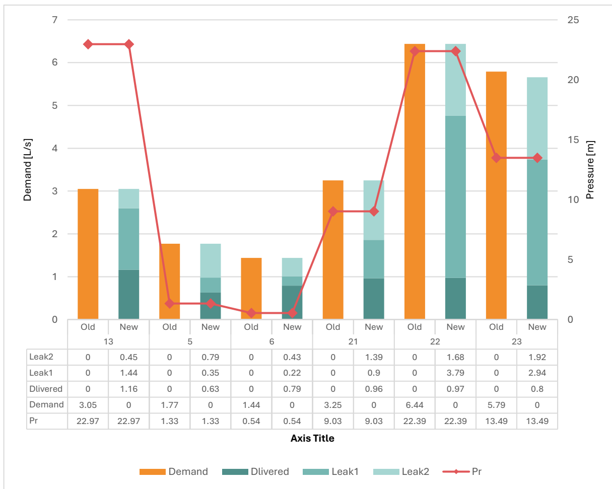
Figure 3-9 Separation of demand for nodes with positive pressure values
