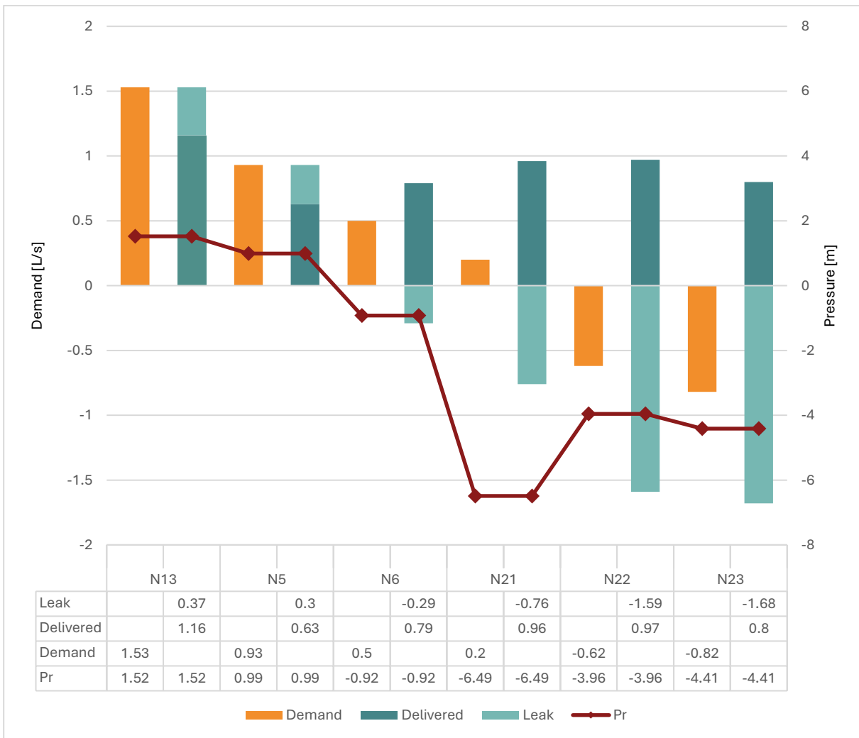
Figure 3-3 Detailed representation of EPANET outcomes (Test-1 with change of elevations)
