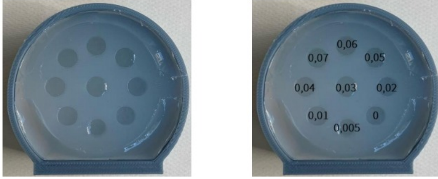
Figure 3.1: Structural image of the phantom containing nine distinct compartments with different concentrations of VivoTrax contrast agent. Each region corresponds to a specific concentration, allowing for the assessment of signal variation and quantitative analysis across a range of known contrast levels.
