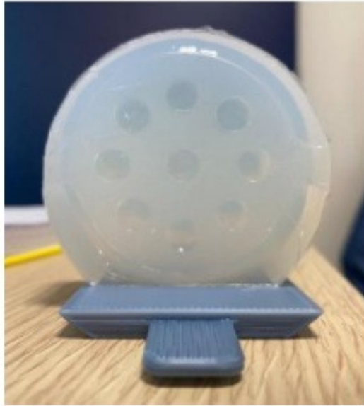
Figure 3.2: Phantom Structure for Positioning. This orientation ensures consistent alignment with the magnetic field and coil setup, minimizing artifacts and allowing for uniform signal reception across all compartments.
