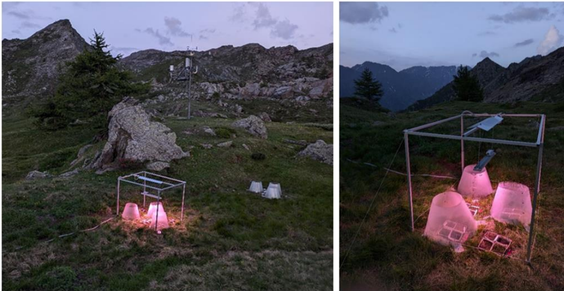
Fig. 12 - the lighting system after the activation of the automatic twilight sensor.
