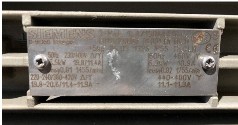
Figure 2.1: Motor parameter nameplate from Manufacturer.
