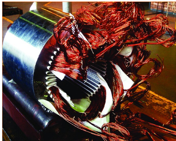
Fig 1.2: Typical Random-Wound Winding being inserted into a stator slot [6].
