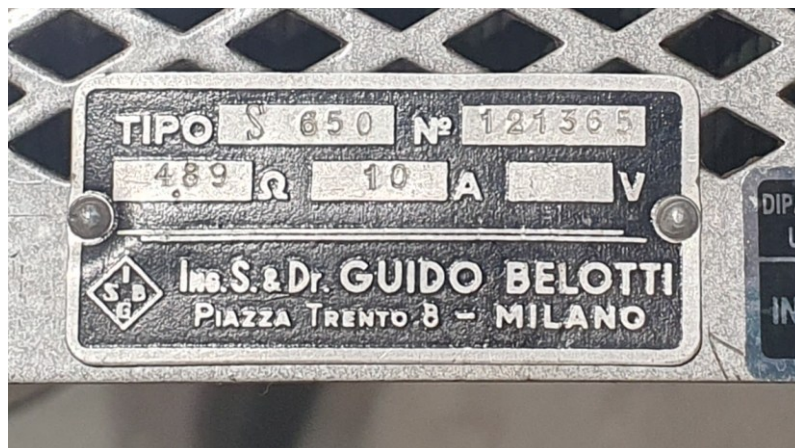
Figure 2.12: A closeup of the rheostat parameter plate.
