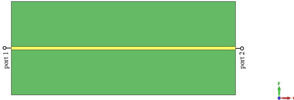
Figure 4-14 Schematic view of the proposed Microstrip Line.
