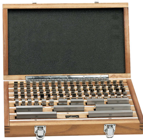
Figure 3.5: Certified Johansson gauge block set used as material length standards during the experimental validation.
