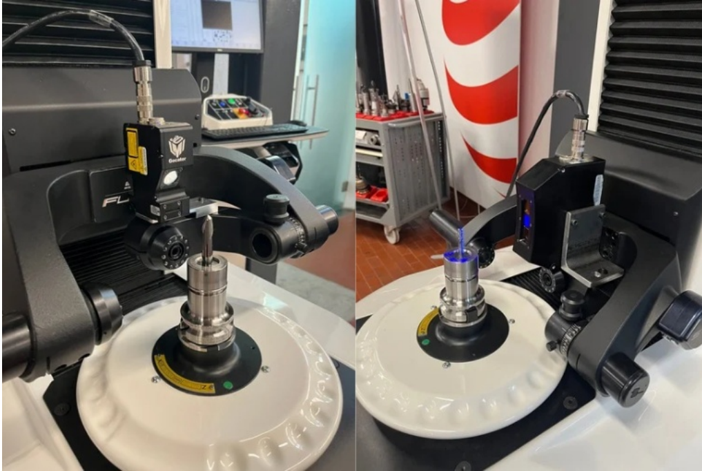
Figure 4.1: Experimental sensor configurations on the Speroni STP FUTURA: laser triangulation (left) and Gocator 3506 snapshot setup (right).
