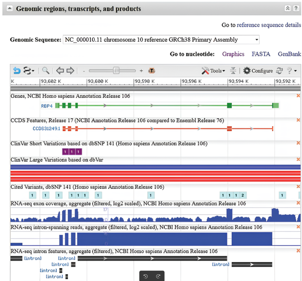
Figure 2.2: View of the annotated location of a gene and its features on a genomic RefSeq. Genomic regions, transcripts and products section of the Full Report. The section for the human RBP4 gene is shown. This is an interactive display of the location of a gene annotated on a genomic RefSeq. More than one genomic RefSeq sequence may be available, and the gene location on any can be displayed using the drop down menu at the top. Zoom and panning functions are enabled, and the tracks displayed can be configured using the “Configure” button. By default, the Genes track displays a merged rendering of transcripts and coding regions. Complete documentation is available by clicking the “?” icon. From NCBI platform. Source: [20].
