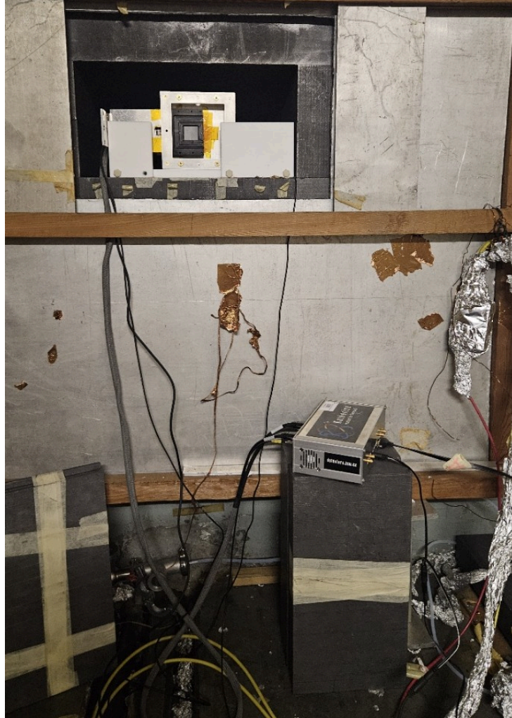
Figure 3.8: Position of the detector in the thermal column. In the image it is possible to see the detector, mounted on the Teflon support, at the edge of the thermal column irradiation room. It is also possible to see where the Katherine readout module was placed due to the cable length issue (the cadmium shielding was removed to take the picture).
